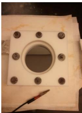
Figure 2: Single-cell set up for etching porous silicon.
